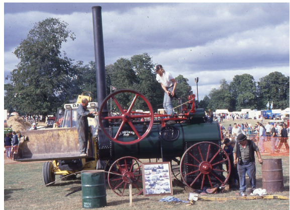
A portable steam engine made by Barrows & Co at the Cherwell Works powering stone crushing machinery at the annual show of the County of Salop Steam Engine Society 2005
