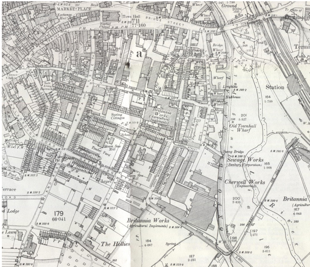
1901 Ordnance Survey map of the Cherwell Street area showing the three parts of the Britannia Works, the Cherwell Works, the factory of W F Lucas & Co and Henry Stone's box factory
